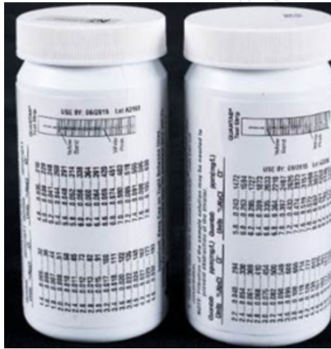
Figure 4. Conversion charts on the back of the Chloride Quantab Test Strip bottle to convert strip reading to chloride ion percentage.
