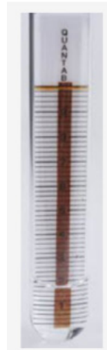
Figure 1. A Chloride Quantab Test Strip in a test solution at the beginning of the test. All Photos in this article are credited to the Government of Canada, Canadian Conservation Institute
