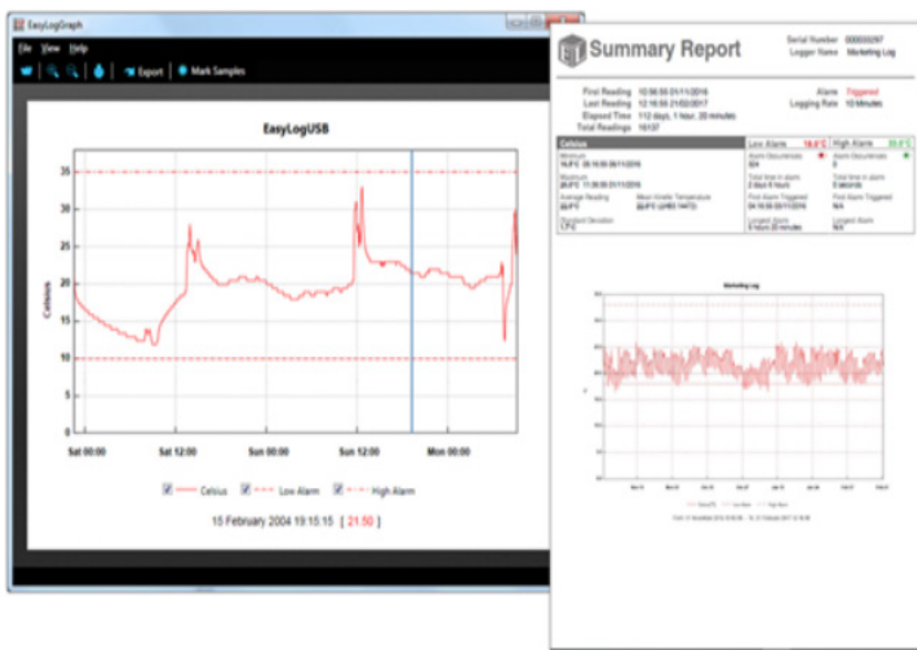
Figure 1. Data report as a graph showing the temperature fluctuation trend over the time period. Photo source: http://www.easylogusb.com/
